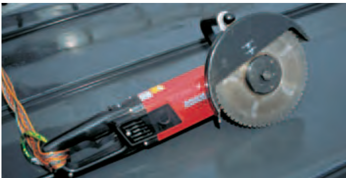
Cutting machine with twin-head rotating cutting discs.
